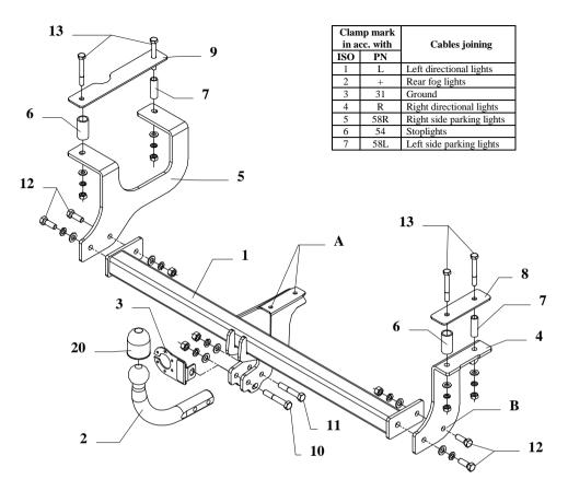
This towbar is designed to assembly in following cars: **SUZUKI WAGON R+** and **OPEL AGILA** produced since 04.2000 till 08.2002, catalogue no. **W14** and is prepared to tow trailers max total weight **1000 kg** and max vertical load **30 kg**.
